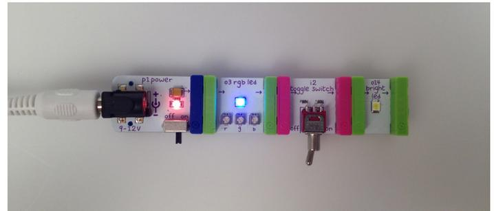
WIRED IN SERIES WITH THE SWITCH ON. THE LED BIT IS OFF.
