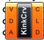
(Curve/Spline/Kinky Curve) Despite its name, a kinky curve is no more than a glorified Interpolated Curve.
