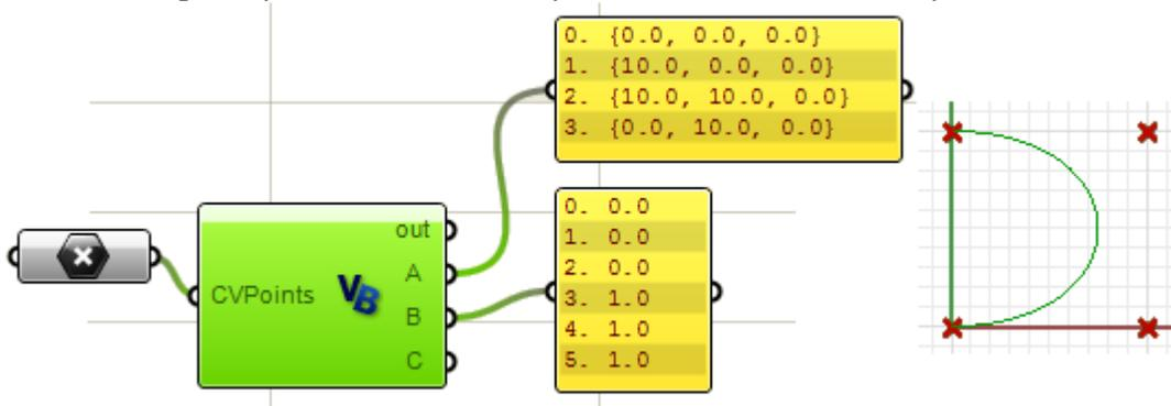
Here is the periodic curve using same input (control points and curve degree):
