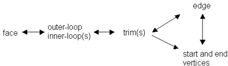
Here is another more detailed diagram of how brep parts are hooked together and how to get from one part o the other.
