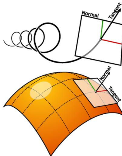
In the case of NURBS surfaces there are in fact two directions implied by the geometry, because NURBS surfaces are rectangular grids of  $\{u\}$  and  $\{v\}$  curves. And even though these directions are often arbitrary, we end up using them anyway because they make life so much easier for us.
