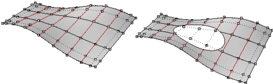
The surface on the left is untrimmed. The one on the right is the same surface trimmed with an elliptical hole. Note that the NURBS structure of the surface doesn't change when trimming.
