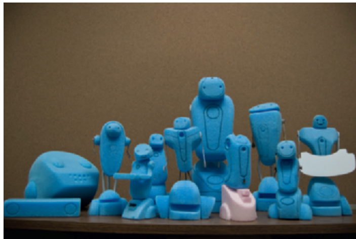
Figure 8.10 Sketches for an interactive robot from Carnegie Mellon’s Snackbot study, which developed a mobile and autonomous robot for delivering snacks to people at Carnegie Mellon University. 30 (Picture by Eric Glaser, thanks to Jodi Forlizzi.)
