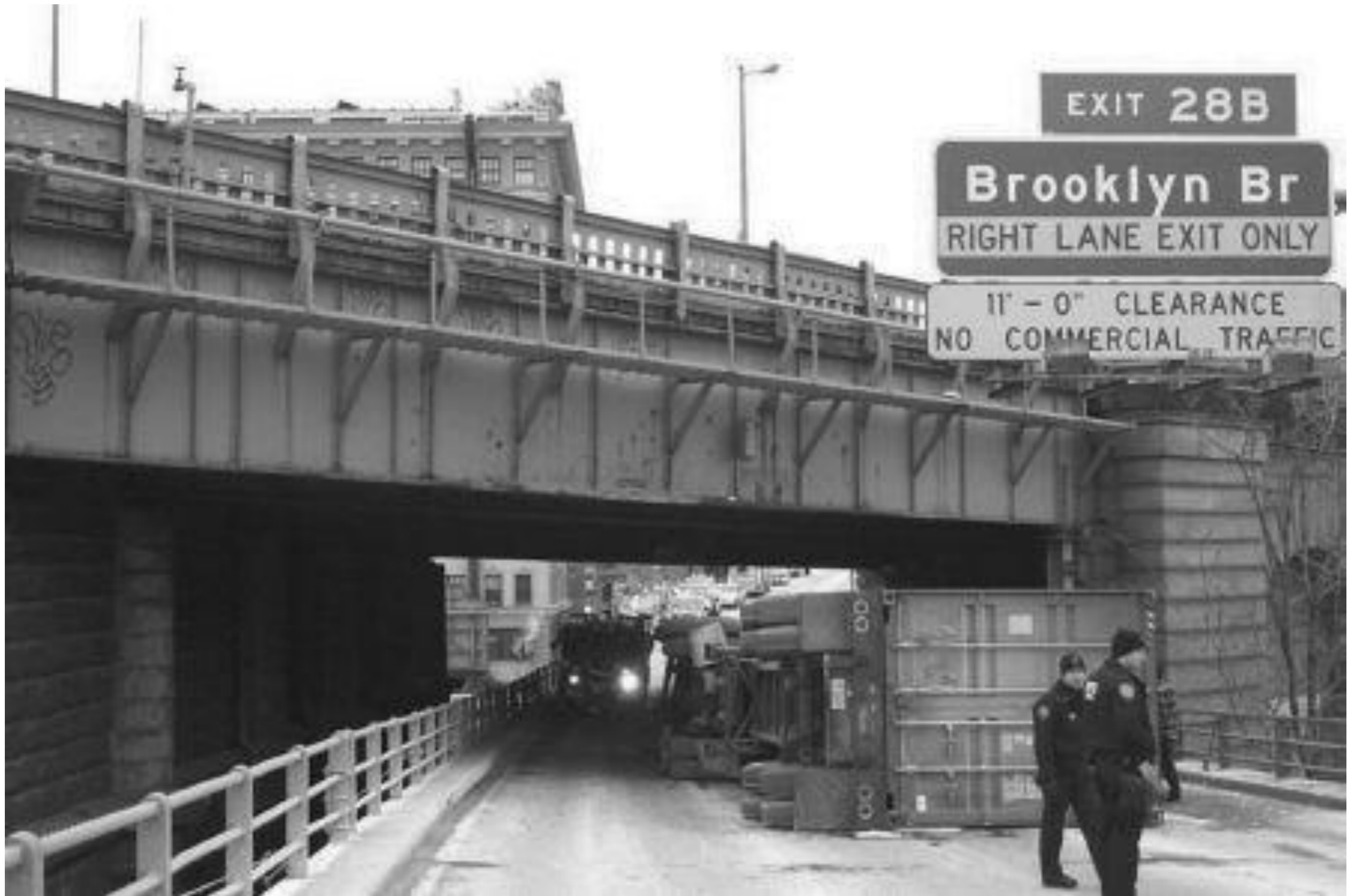
Low overpass. Oversized overturned truck on the BQE under the Brooklyn Bridge. Photo: B. Yanev, NYC DOT.
